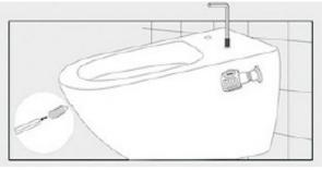
8. Once the installation is completed, a flush and leak test should be carried out and once it has been commissioned, the toilet can be sealed around the edge to finish.
